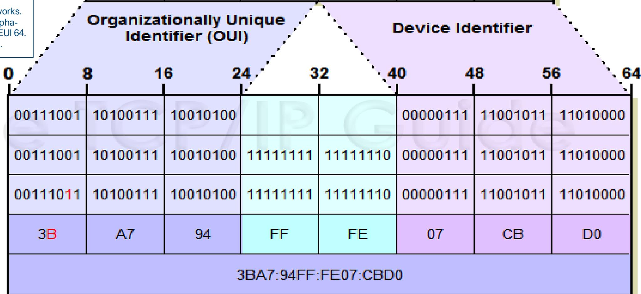
**64-Bit IPv6 Modified EUI-64 Interface Identifier**
