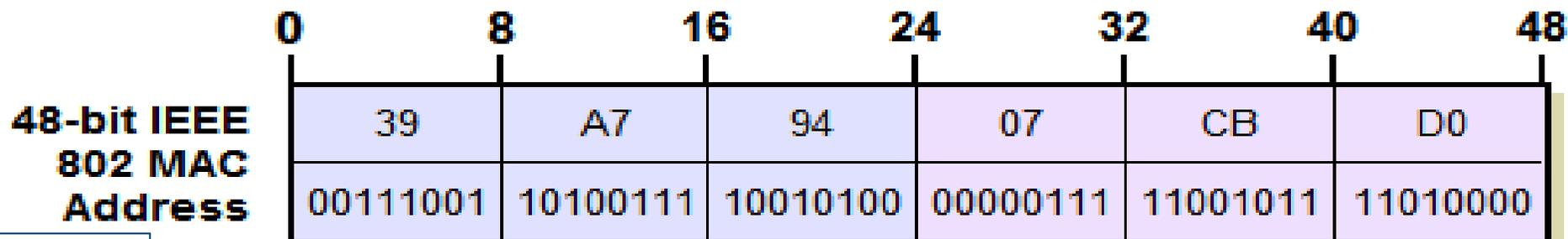
This is how SLACC without DHCP works. Uses a random generated 64 bit alphanumeric number combined with the EUI 64. Creates a 128 bit IPv6 address.
